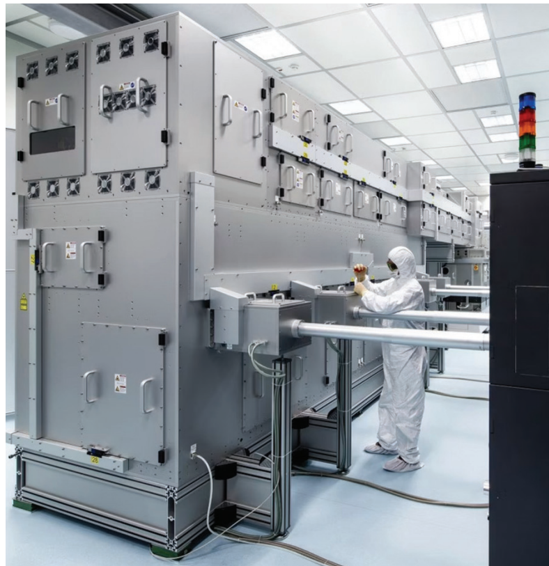
LineBeam system that performs low-temperature laser annealing of polysilicon backplanes for OLED and LCD high-resolution displays. The system can use either 355-nm or 308-nm excimer laser beams depending on the material annealed.
