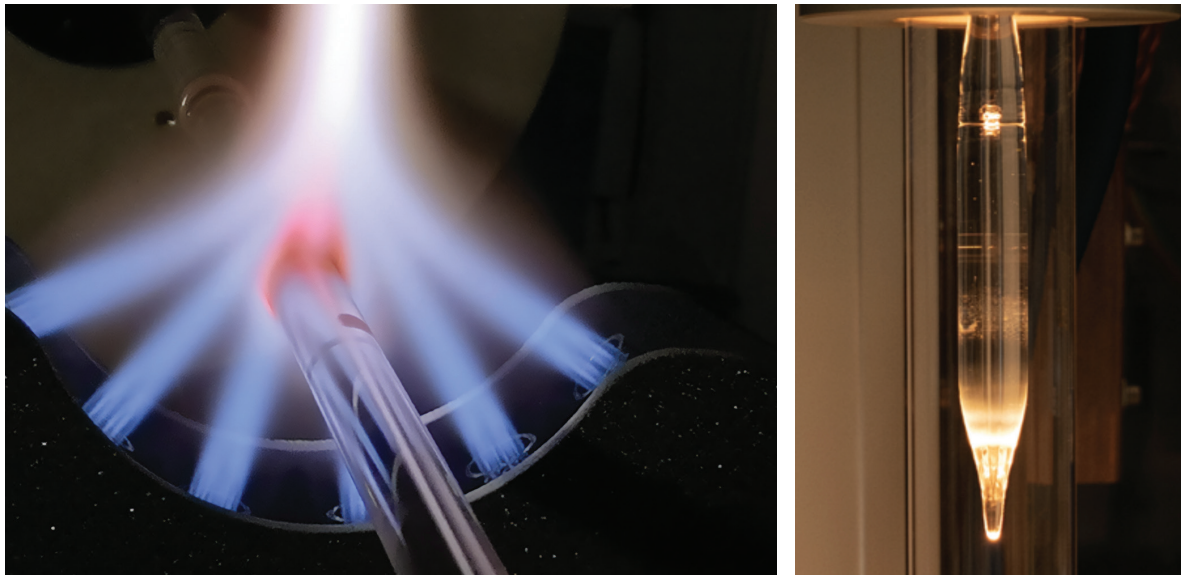
Examples of hollow-core fiber during the manufacturing process.
