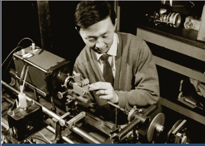
Charles K. Kao measuring the transparency of fused silica at STL in Harlow, UK. [Nortel and BNR Europe / Courtesy of J. Hecht]
