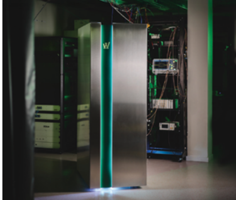
Welinq, which the authors cofounded, in 2025 released QDrive, an industry-grade racked quantum memory with a 90% storage-and-retrieval efficiency and >99% fidelity.
