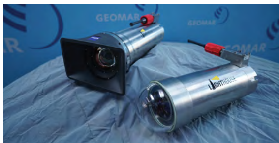
Top: GEOMAR's "Lighthouse"—which combines a new cinema-quality camera co-developed with Carl Zeiss, additional cameras, high-intensity LED strobes, acoustic sensors and laser ranging—mounted on the ROV Phoca for a mission in Sogn Fjord, Norway. Bottom: Cameras of the Lighthouse system.
