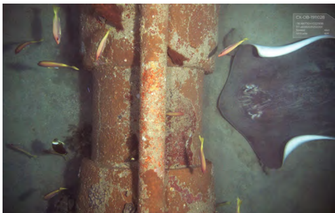
Left: Cathx Ocean’s Hunter II system includes a 510–530-nm laser, an optical camera, a laser camera and banks of bright pulsed LEDs. Right: Hunter II image of a section of pipeline, taken 4 m above the seafloor in an AUV traveling at a relatively fast 4 knots, shows substantial detail without motion blur.
