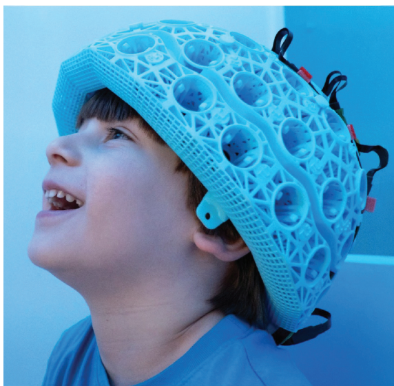
A 3D-printed helmet that uses quantum sensors to measure human brain function.
