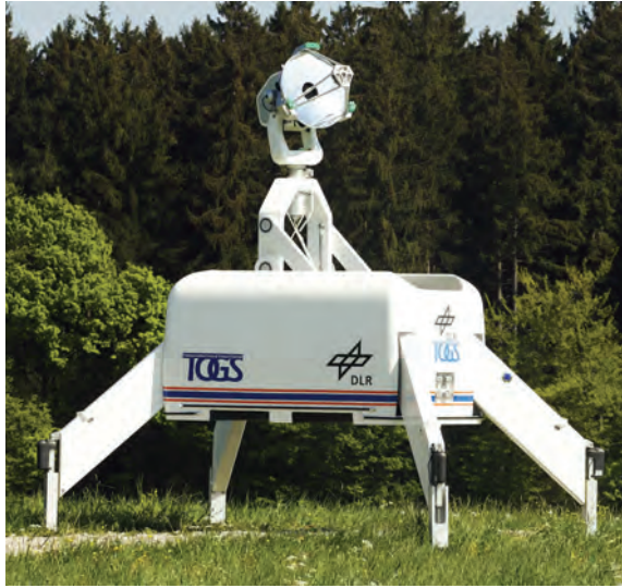
The Transportable Optical Ground Station operated by DLR, which can be deployed globally in its cargo-sized container. ESA
