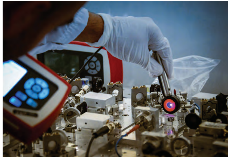
A quantum engineer measures the optical power of a laser beam at Atom Computing’s research and development facility in Boulder, CO, USA.
