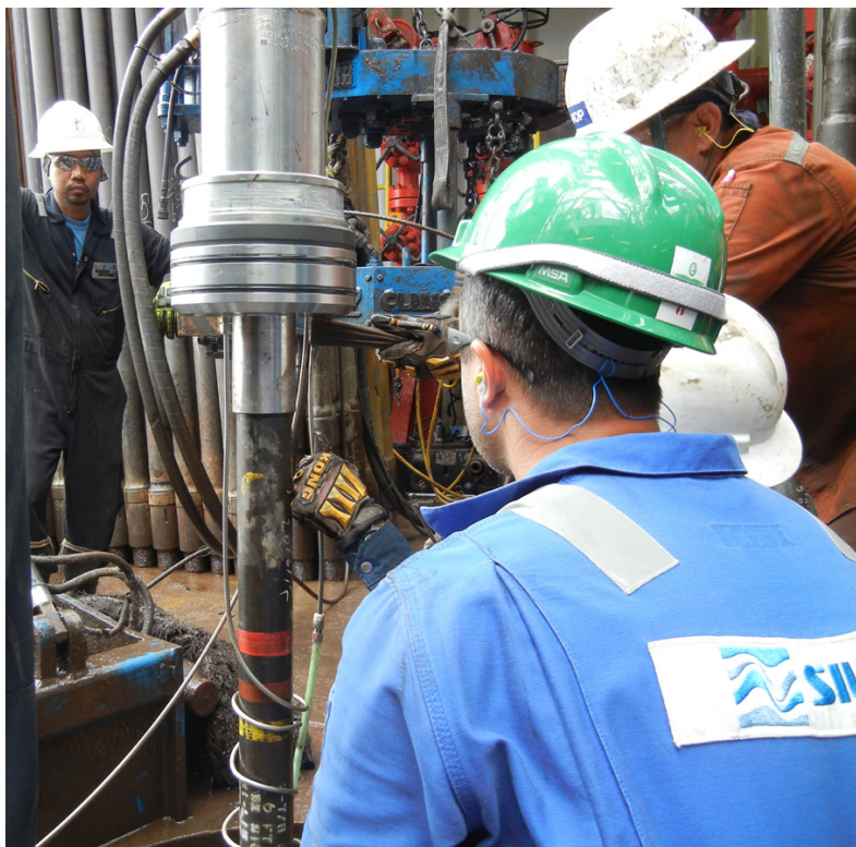
Fiber optic cables are sent down deep wells to gather data during seismic surveys of oil and gas deposits. The fibers, which measure stress and temperature via Rayleigh scattering, can take data along their entire length. Silixa Ltd.
